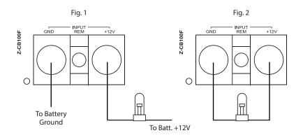
Note: The bulb has no polarity so it does not matter which side is connected to the capacitor or the battery. The bulb can get extremely hot and should not be touched or handled until it has cooled.
